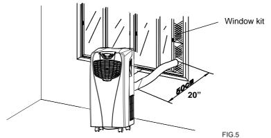
1. Open the window and insert the window kit to cover the open gap. Next, slide the window across so that the kit is held securely. You may need to adjust the size of the window kit and secure it with screws. This technique may also be used for sash windows.
